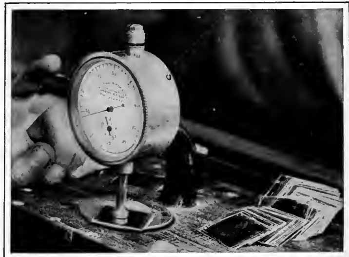
IN THE MANUFACTURE OF FIXED CONDENSERS The mica must be accurate in thickness. One degree on the large-scale micrometer in the photograph equals one one-thousandth of an inch
